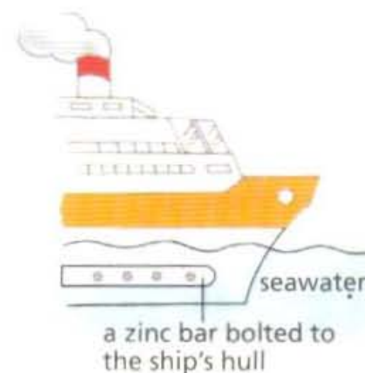
Fig 14.22 Rust prevention using a sacrificial metal
