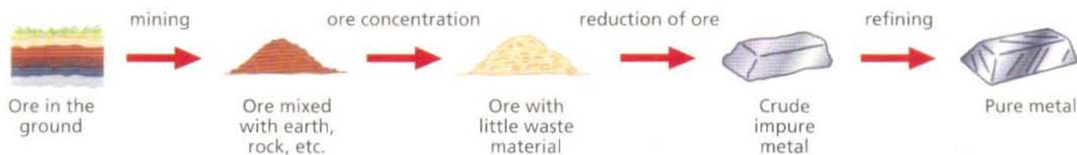
Fig. 14.15 The stages involved in obtaining metals from their ores
