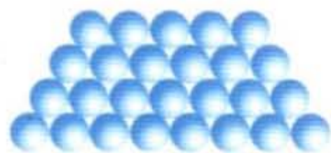
Fig. 14.1 A simple model of the structure of metals
