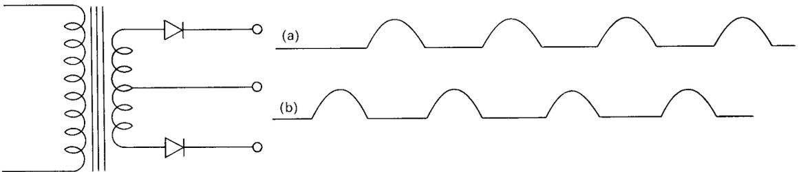
If the two outputs are connected in parallel, the combined output is as shown below. Such an arrangement is known as *full wave rectification*.
