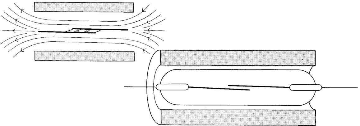
An attractive type of relay for switching small currents very quickly and reliably is the reed relay. It consists of two iron reeds inside a sealed tube, usually filled with an inert gas to avoid corrosion of the contacts. The tube is
