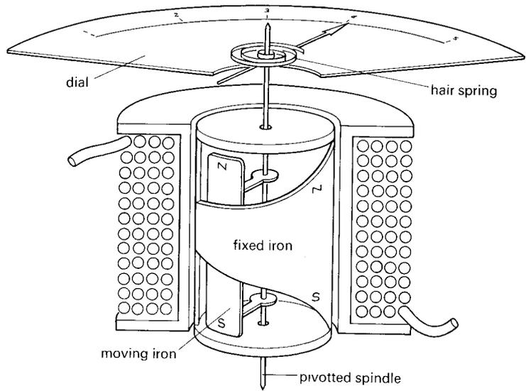
record the current after it is switched on, since it overshoots the mark and moves backwards and forwards many times before finally coming to rest. Better instruments have some form of 'damping' to reduce these oscillations: for example, a light vane can be attached to the moving part to increase air resistance.
