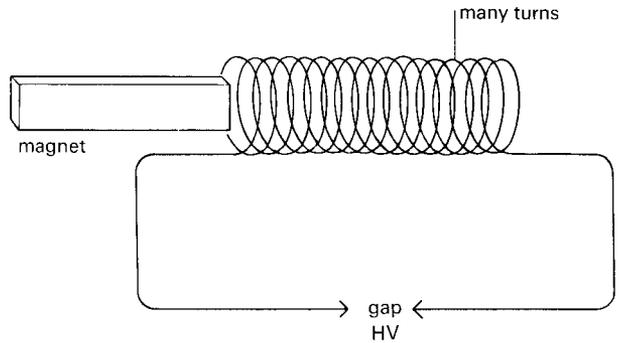
the voltage might be high enough to make a spark jump a gap of a millimetre or so. In practice, it is easier to obtain the effect of removing the magnet quickly by electrical means.
