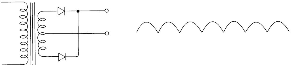
Devices of this sort are used whenever direct current is needed and the normal a.c. mains is available. Such a voltage supply used in schools is shown on the opposite page. You may also use one for supplying a toy electric rail-
