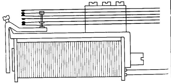
When the current flows through the coil, it magnetises the iron core and attracts the armature. The top end of the armature is raised and closes the switch contacts by pressing against them. Thus a current in the coil can switch on a current in another circuit.
