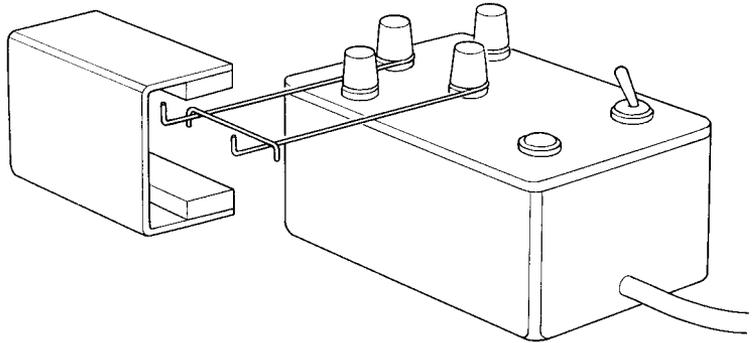
A wire was put between the poles of a magnet. When a current flowed through the wire, there was a force on the wire at right angles to both the current and the magnetic field. The wire was not attracted to the poles: it was pushed in or out depending on the direction of the current.
