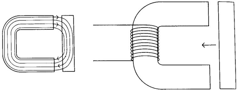
The smaller the gap between the magnet and the iron, the bigger the force of attraction. It is important to realise that if one needs a big force, the design of the device should keep this gap as small as possible.
