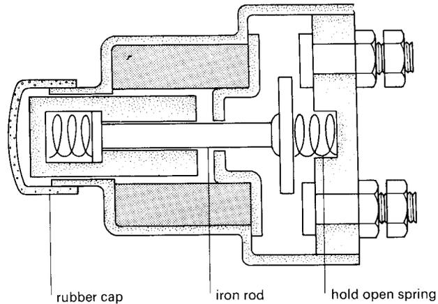
The illustration above shows yet another arrangement: the armature this time is the iron rod inside the coil. It is spring loaded so that normally there is a very small gap, but, when a current is passed through the coil, the armature moves, thereby engaging the moving contact with the fixed contacts.
