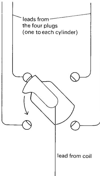
distributor cap is also made of a high quality insulating material, as is the rotor arm.
