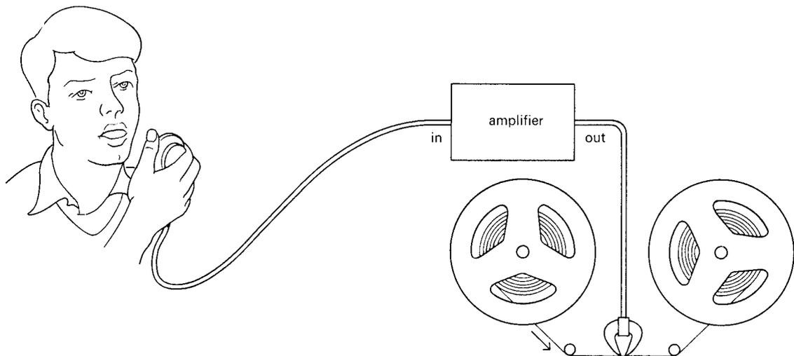
fier is necessary to increase the weak currents from the microphone to large enough currents to imprint a magnetic pattern on the tape as it goes past.
