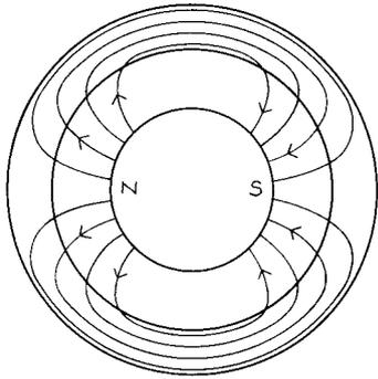
A cheaper and more convenient magnetic field for such instruments which is becoming increasingly popular is shown on the left. In this the core is a permanent magnet in the form of a cylinder, magnetised across a diameter. This is surrounded by a cylinder of iron which is such that the magnetic field in the gap is very similar to that shown on the left.
