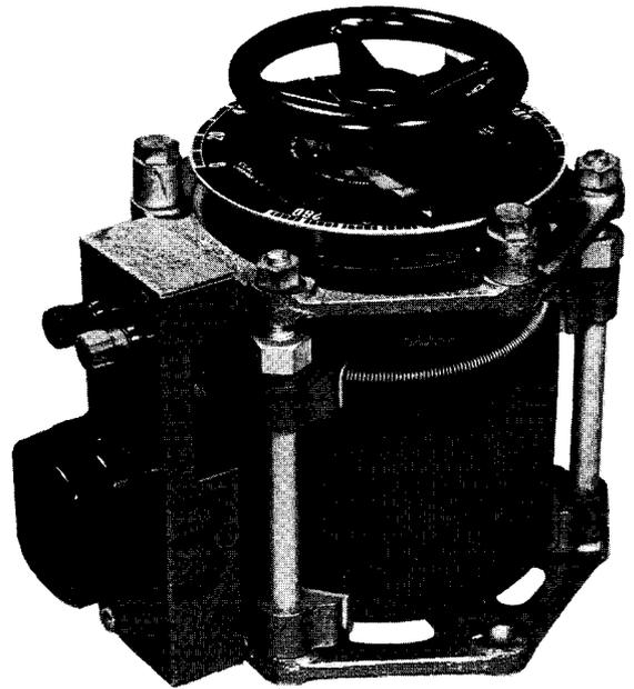
The primary coil is wound round an iron ring: the form of winding is called a *toroid*. A brush moves round, making contact with this coil so making a variable tapping similar to that in the auto-transformer, but enabling the output voltage to be adjusted between 0 and the full mains voltage.
