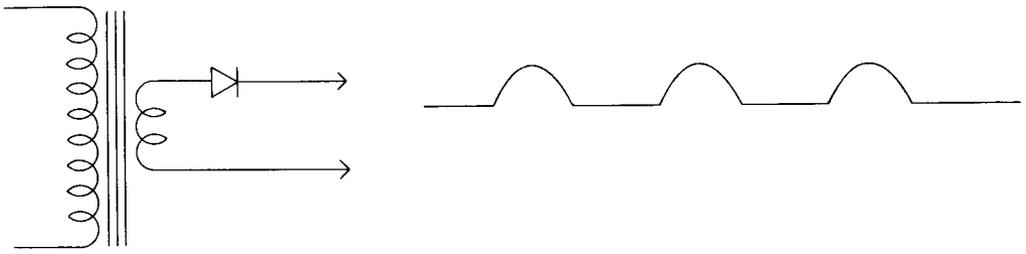
In the arrangement above the transformer steps down the voltage from 240 volts to 1 volt. The secondary coil is connected through a rectifier to the output terminals. The output voltage varies with time as shown: the negative half of the alternating voltage being cut off by the rectifier which conducts in one direction only.
