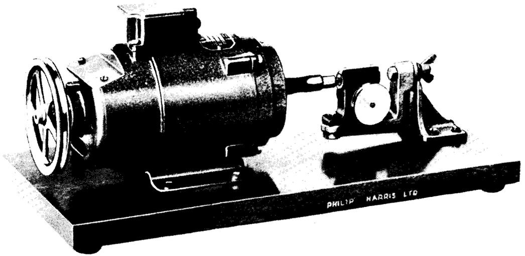
*Fractional horsepower motor*
