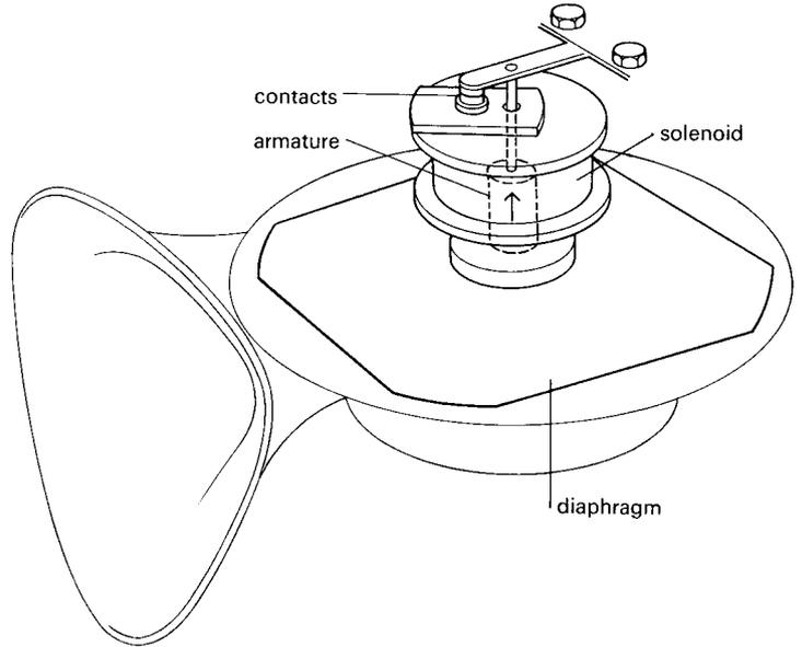
You can see in the diagram that, as the armature is attracted in to close the gap, it simultaneously presses open the contacts, thus switching off the coil current. The armature falls back, contact is again made and the process is repeated just as in the electric bell, but at a very much higher frequency.
