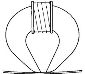
Notice that there is a very small gap. A piece of the tape resting across this gap would be magnetised, one way or the other, when a current passes through the coil. Suppose the tape was moving and an alternating current
