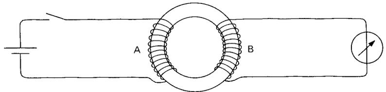
magnet: it is equivalent to putting a magnet into coil B; a burst of current flows in the second circuit. When the first circuit (the primary circuit) is switched off, it is equivalent to removing the magnet from coil B; a burst of current flows in the opposite direction. A current could be made to flow backwards and forwards in the secondary circuit by switching on or off the current in the primary.
