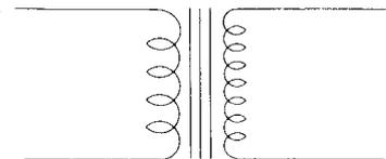
The usual electrical symbol for a transformer is shown on the left, the primary and secondary coils and the iron core being symbolically represented.
