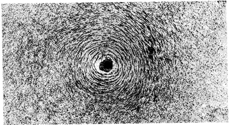
*Field due to a current in a long straight wire*
