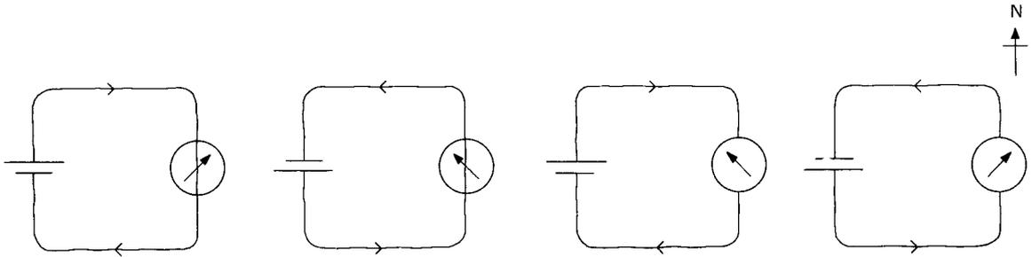
A wire passing North and South above a compass needle caused the needle to be deflected either towards the East or the West according to which way the current was flowing in the wire. The needle was deflected in the opposite directions when the wire was below the compass needle.
