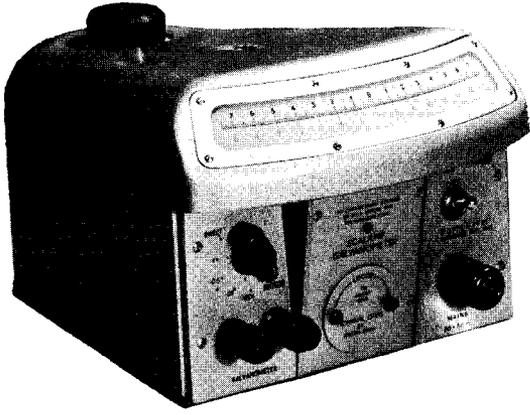
As the suspension is very weak, it is impracticable for it to support a pointer. Instead, a small mirror is fixed to the coil. A beam of light falling on the mirror is reflected on to a scale. As the coil rotates (winding up the phosphor bronze strip) the spot is deflected to a new position on the scale. Because of the distance the beam of light travels, it is equivalent to having a very long pointer.
