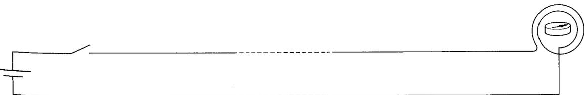
The circuit of such an elementary system is shown above. When someone at the source switches on or off, the galvanometer at the distant point indicates this fact.
