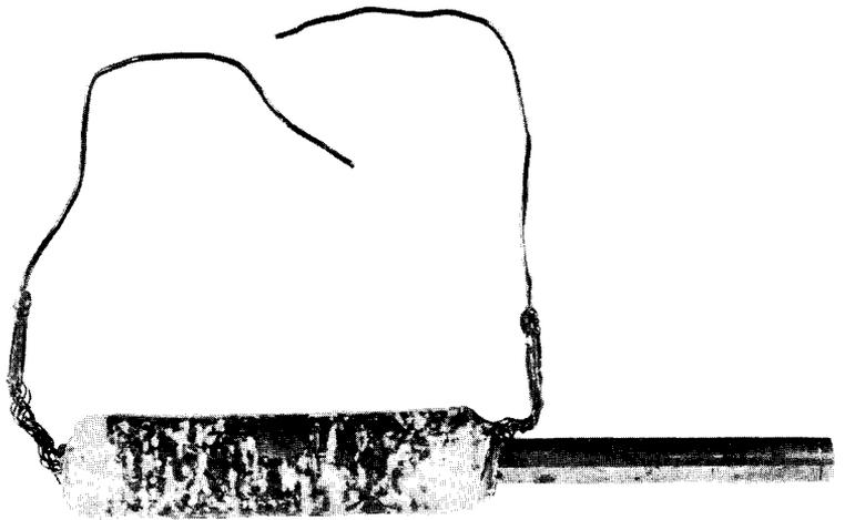
What Faraday has shown may be briefly summarised as follows. If a magnetic field through a coil is *altered*, a voltage is induced across the coil which will cause a current to flow in the circuit connected to it.
