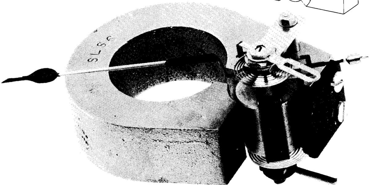
A coil is arranged on pivots so that it can be rotated about the cylinder with the sides of the coil in the gaps. Connections to the coil are made through the hair springs which keep it in the zero position when there is no current flowing.
