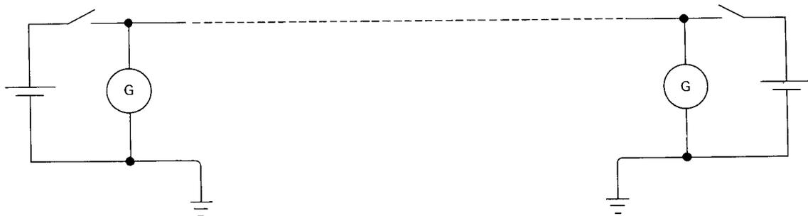
Of course the detectors at both ends in the above circuit will operate together. Can you think of a way of switching in which only the distant detector works when the switch or key at the home station is pressed? In the circuits above, the detectors were galvanometers, but they could be replaced by buzzers if the current is great enough.
