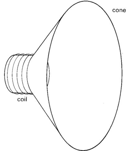
The coil is attached to a cone several inches in diameter. An alternating current through the coil will drive the coil and cone in and out. This will set into vibration a large mass of air because of the size of the cone. Thus, if the electric current has a frequency of 256 Hz, the loudspeaker cone will vibrate 256 times per second and a middle C will be heard.
