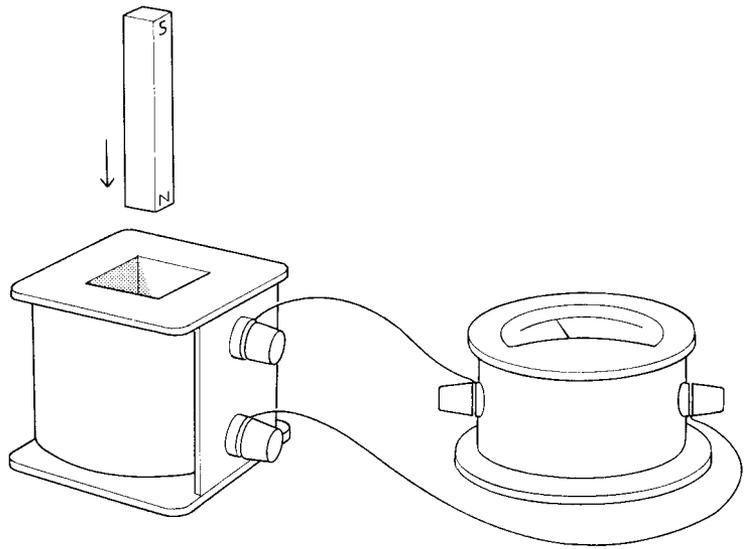
No current flows in the galvanometer. But if a magnet is put into the coil, the galvanometer needle moves. The current ceases once the magnet is inside. When the magnet is pulled out, a current flows momentarily in the opposite direction. You probably also noticed that the faster the movement, the greater the deflection.
